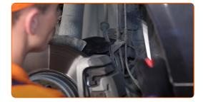
Separe o conetor do sensor ABS.
