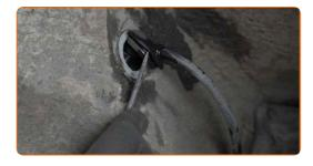
Separe o conetor do sensor ABS.
