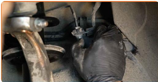
**84** Junte o conector do sensor ABS.
