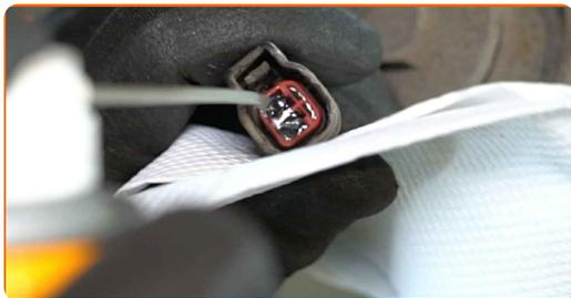
**69** Junte o conector do sensor ABS.
