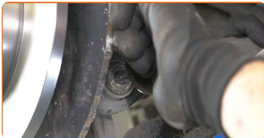
**20** Separe o conetor do sensor ABS.
