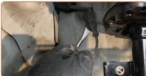
**20** Separe o conector do sensor ABS.
