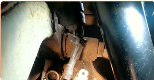
**9** Separe o conector do sensor ABS.
