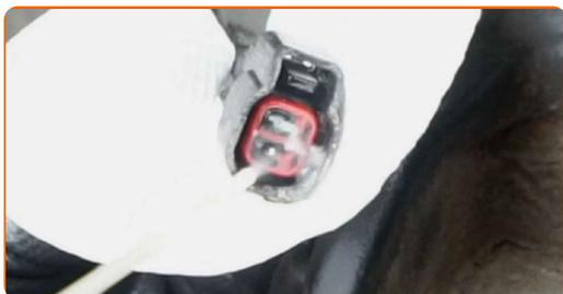
**68** Junte o conector do sensor ABS.
