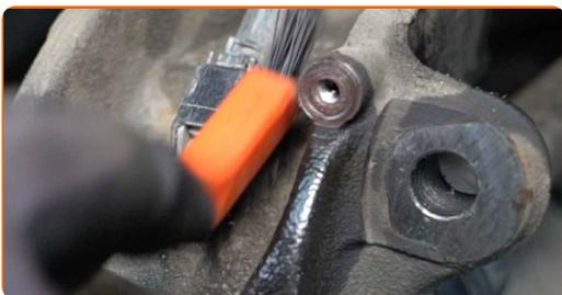
**26** Separe o conector do sensor ABS.
