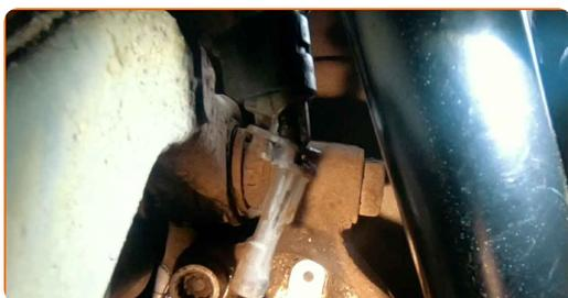
9 Separe o conector do sensor ABS.
